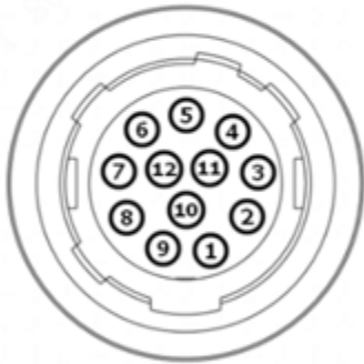
Port definitions of 12-pin signals
