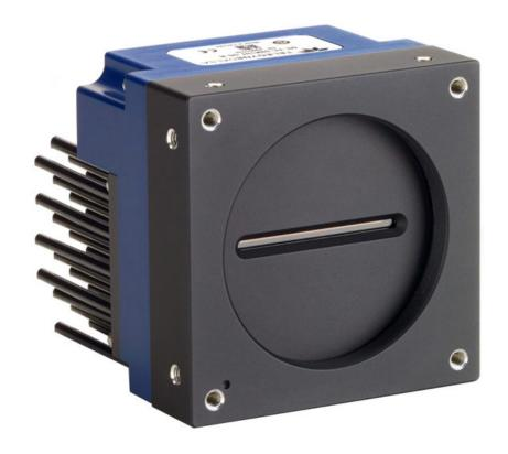
The Linea ML brings leading edge CMOS technology that is faster than ever, with affordable multiline architecture that enables the newest, most powerful inspection techniques including HDR, color and multispectral analysis, and multifield imaging (single-pass bright/darkfield). With a native fiber optic interface for easy, low-cost long distance cabling, Linea ML opens new horizons in inspection.
